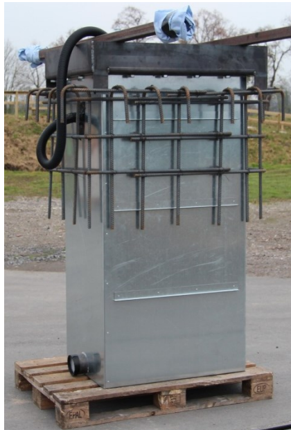
Picture 8: Bollard with reinforcement fastened to metal housing
