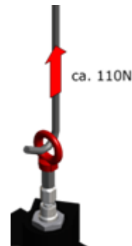
Picture 22: Solenoid valve with manual override and tool for emergency lowering
