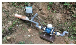
Measurement of a spring discharge with battery-powered Promag W 800
