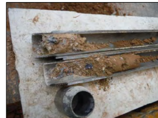
Foto 11: Sondeig S-3, SPT a 7,0 metres.
