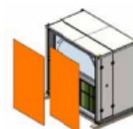
Step 3: Remove 2 Alkilux plates and set of 5 screws M8 and 2 corner elements
