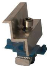
Final Clamp Set of parts including a captive nut, end support clamp, M8 hex socket screws, head notched on the underside.
