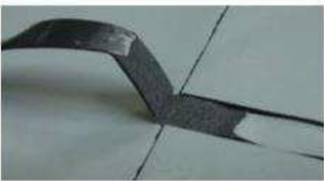
Pull from each side of the weld
