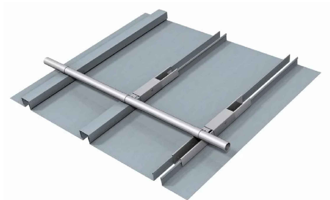
DETALL TUB PARANEUS Ø50mm
