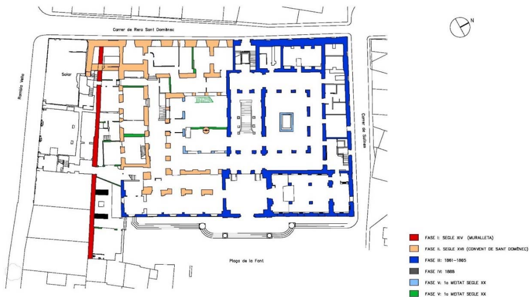
Figura 13. Diferents fases constructives Palau Municipal
