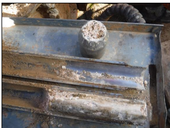
Foto 3: Sondeig S-1, SPT a 4,0 metres.
