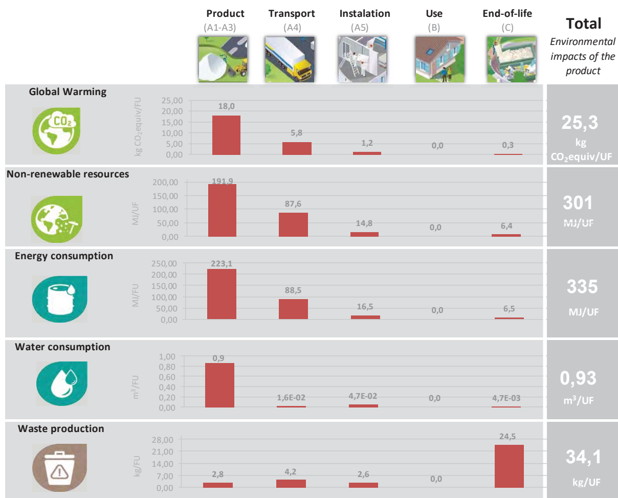
Environmental impacts of SATE System with TF Profi insulation
