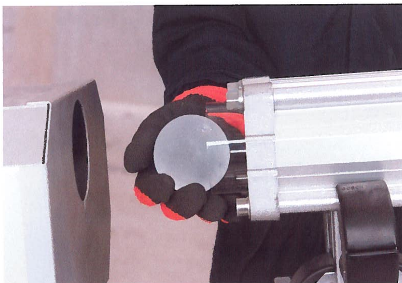
Illustration 2: loading of the equipment, with a laboratory made, transparent, ice ball (70 mm diameter)
