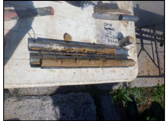
Foto 8: Sondeig S-2, SPT a 5,0 metres.
