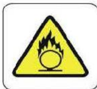
SA-020 IPELIGRO! MATERIAL COMBURENT
