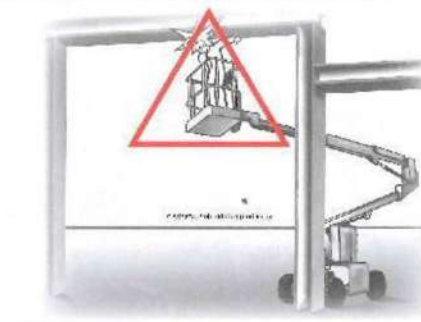
16.- RADIUS OF ACTION Check and eliminate any obstacle that hinders moving or raising the platform and leave enough free space above head.
