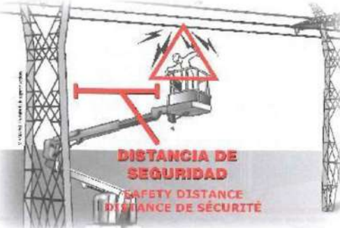
18.- POWERLINES It is indispensable to maintain a safe distance from any powerlines.
