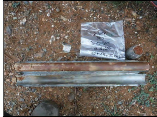
Foto 2: Sondeig S-1, SPT a 1,0 metres.
