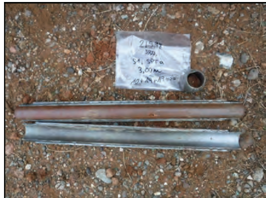
Foto 3: Sondeig S-1, SPT a 3,0 metres.
