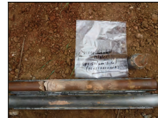
Foto 23: Sondeig S-7, SPT a 3,0 metres.
