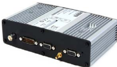
Figura 1: CPU terminal RESCAT
