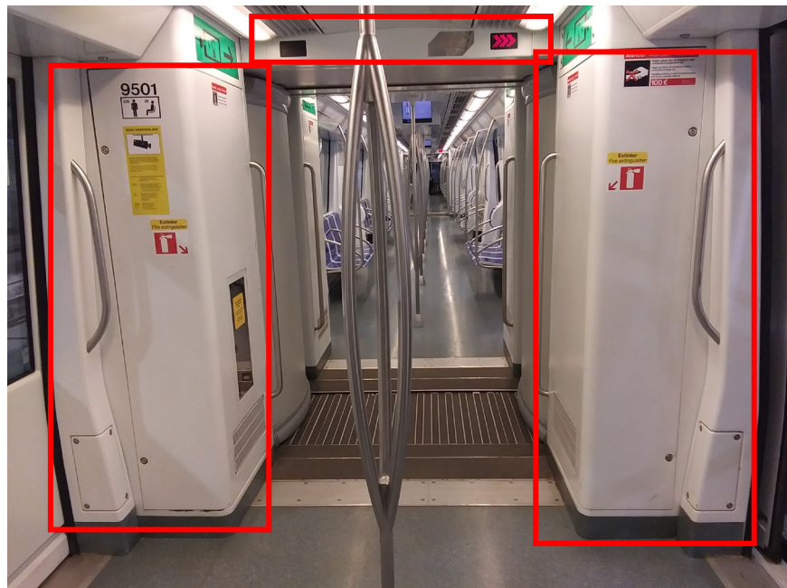
Figura 3.7. Revestiments testera inter vehicular S/9000
