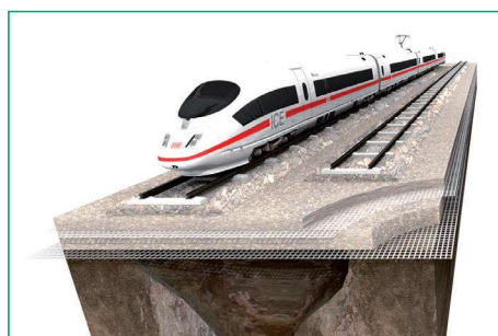
Figure 8 Secugrid® soil reinforcement in railroad applications
