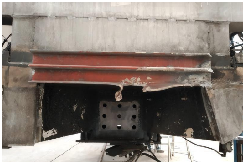
Figura 13: Anticlimber central, danyat
