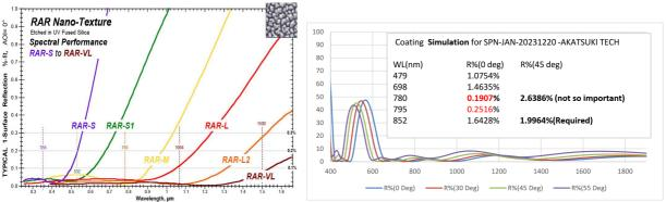
**Left**: Reflection values of different RAR coatings. The y-axis spans a range of only 1%. The figure is taken from TelAztec's webpage. **Right**: Simulated reflection values of a thin-film coated, provided by Akatsuki upon request.
