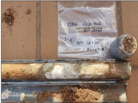
Foto 15: Sondeig S-4, SPT a 1,0 metre.
