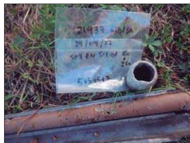
Foto 2: Sondeig S-1, SPT a 2,0 metres.
