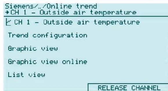
Figure 10-5 Setting trend parameters and defining the view
