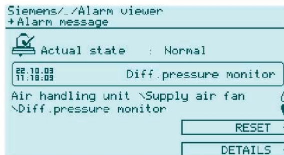
Figure 7-5 Example of Extended alarm
