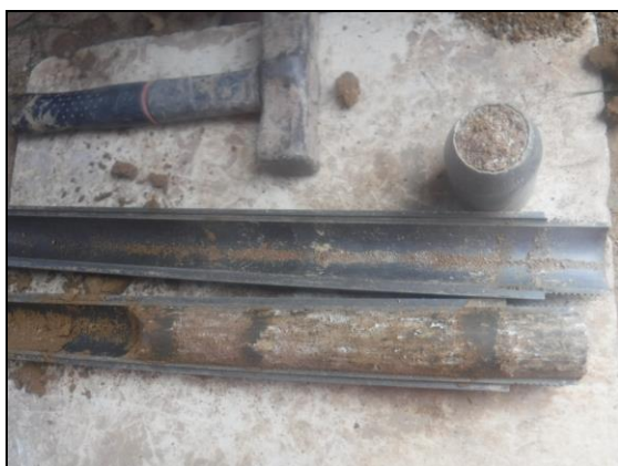
Foto 17: Sondage S-4, SPT a 6,0 metres.
