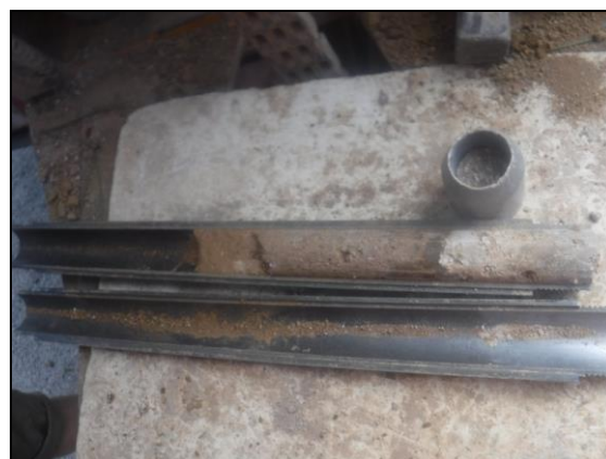
Foto 16: Sondage S-4, SPT a 3,0 metres.
