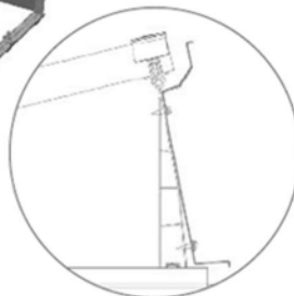
Simple alignment (e.g. southward), incline: about 13° with Windsafe sheets for ballast optimization
