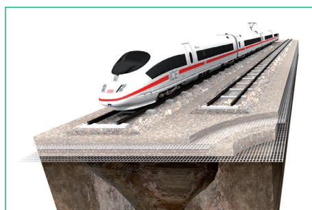
Figure 8 Secugrid® soil reinforcement in railroad applications
