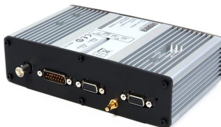
Figura 1: CPU terminal RESCAT
