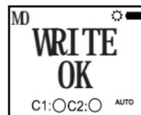
**WRITE OK** : It indicates that all the information on the DTR-IR Prog has been successfully transferred to the DTR-20M device. When this message is displayed, Green LED of the DTR-IR Prog will turn on.
