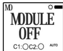
**MODULE OFF** : After removing power from the device for 3 seconds, MODULE OFF message will be displayed. This message indicates that communication module is off and DTR-IR Prog can't be used.
