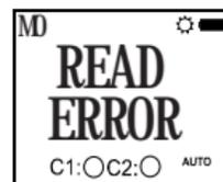
**READ ERROR** : It indicates that the data transfer from DTR-20M to DTR-IR Prog wasn't successful because of an interruption of the visual connection or because of the long distance between two devices. When this error is displayed, all data read by the DTR-IR Prog up until that point is discarded. Previously saved values on the DTR-IR Prog aren't deleted. When this message is displayed, Red LED of the DTR-IR Prog will turn on.
