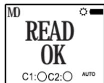
**READ OK** : It indicates that all the information on the DTR-20M device has been successfully transferred to the DTR-IR Prog device. When this message is displayed, Green LED of the DTR-IR Prog will turn on.
