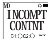
**INCOMPT CONTNT** : The data on the DTR-IR Prog device can only be transferred to a DTR model which the data is programmed for. If you try to transfer the data from the DTR-IR Prog device to an incompatible DTR device, this error message will be displayed. But you can read the content of any DTR device. This way, the data on the DTR-IR Prog device will belong to the appropriate DTR device.
